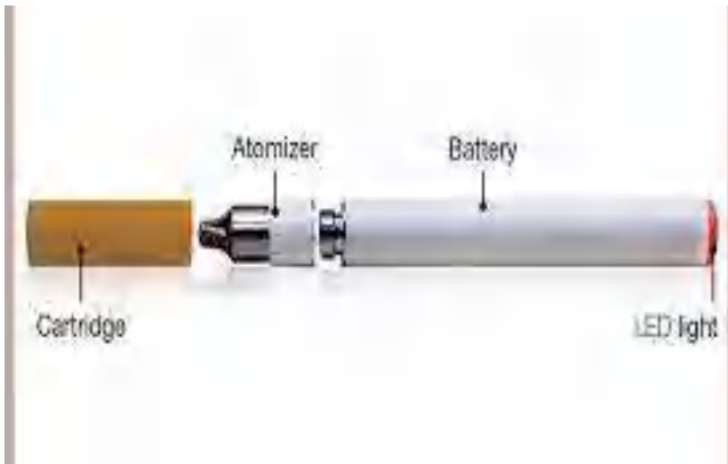
Fig. 2 Structure of a standard electronic cigarette
